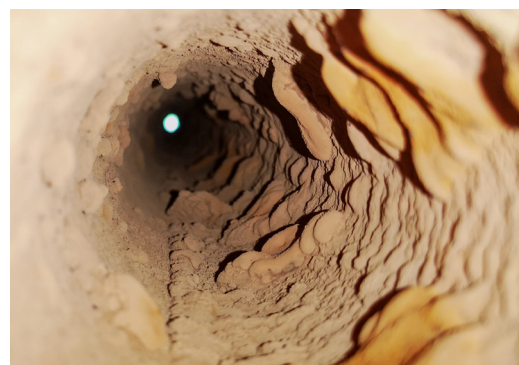
Limescale build-up inside lavatory pipes
