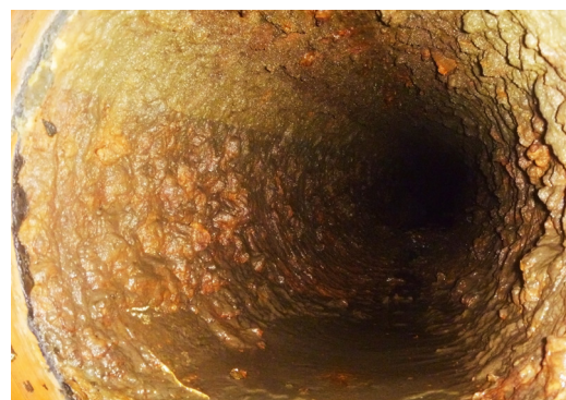
Limescale build-up inside lavatory pipes
